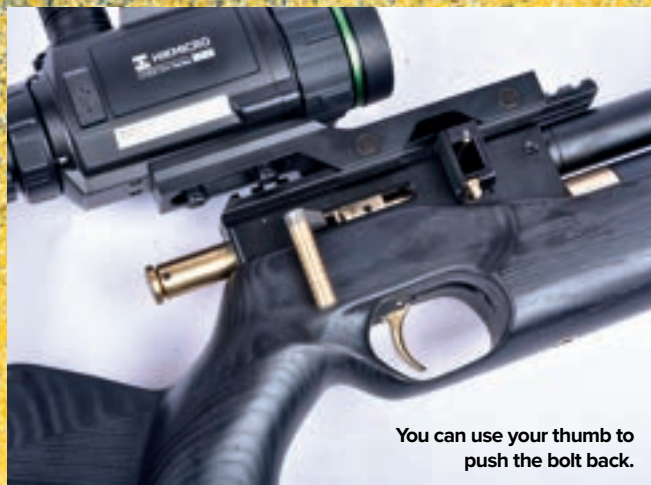
When you pull the lever back the bolt pushes out.
