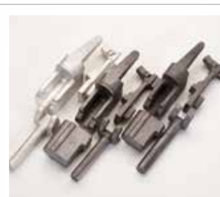
Basculi, sottoguardie, croci e monoblocchi ricavati da masselli forgiati Action bodies, trigger plates, iron fore-ends and barrel extractors pieces are milled from forged steel ingots. Basculas, sous-gardes, monoblocs et lonquesses usinés à partir de blocs forgés
